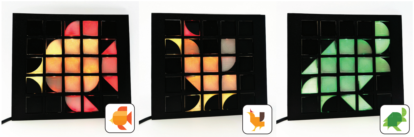
Fig. 1. Diceplay , a modular physical canvas for abstract visual composition. Diverse abstract designs automatically generated by our optimization framework are physically realized using a low-power, LED-enabled dice display, which can be reconfigured through changes in dice orientation and dynamically updated via programmable color.
